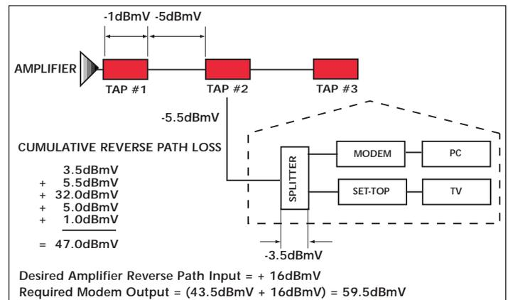
Figure 3. This example shows added attenuation losses of 3.5dBmV due to 2-Way Splitter addition for connection of cable modem.
