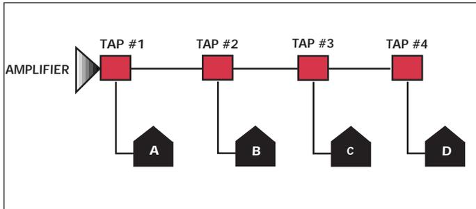
Figure 1. The RF signal level at the entry point to each home must be approximately 7dBmV. The coupling values of Taps 1 through 4 are chosen to ensure this consistent RF level at each home entry port.
