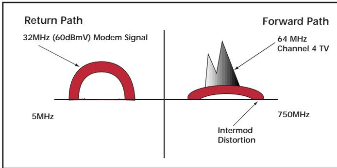
*Figure 5. This example shows a return path signal that is being transmitted at 32MHz. As the ferrite saturates, due to the high level signal being transmitted, a second harmonic beat will appear at 64MHz (twice the fundamental frequency).*
